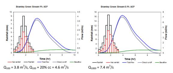
4.13 The 1% AEP flows are reproduced in tabular form below, together with an allowance of 20% for climate change and the 0.1% AEP flows.
